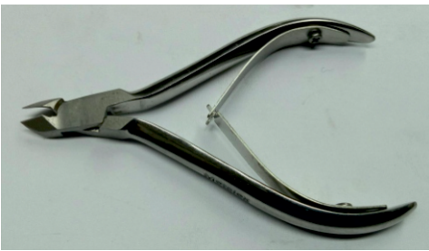
Article No 27-145 nail nipper 10 cm/ Tip 7mm, lap joint double spring steel grade AISI J 420 / Satin finish, Hardness 49 to 51 HRC
