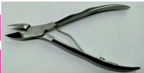
Article No 27-40 nail nipper 10.5cm/ Tip 12mm, lap joint single spring steel grade AISI J 420 / Satin finish, Hardness 49 to 51 HRC
