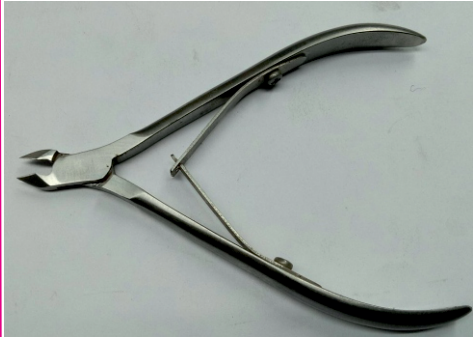
Article No 27-148 nail nipper 10 cm/ Tip 5mm, lap joint double spring steel grade AISI J 420 / Satin finish, Hardness 49 to 51 HRC
